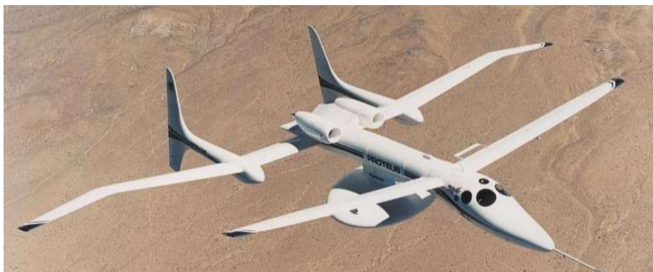
Fig. 7 HALO Proteus aircraft. Note the pod for the payload underneath. (Courtesy of Angel Technologies Corp.)
